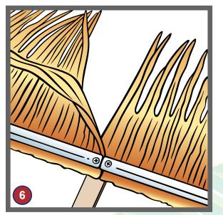
6) At a rail junction, you must create an **overlap** of a minimum of 5 cm (2") between the leaves on the new rail to the leaves already installed on the first rail.
