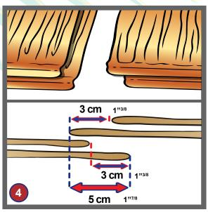
4) For the first two rows: insert a double layer of leaves with a 3 cm (1 " ½) overlap on the rail.
