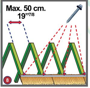
Fix rails to vertical battens. Space between battens must be a maximum of 50 cm (19"5/8).
