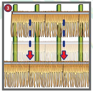
3) **IMPORTANT:** As you start a new row, the new row of leaves must start half way along the leaf below (like brick-laying). Therefore, every other row starts with only a half leaf to fill the gap.
