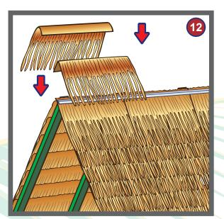
12) For extra protection against **water infiltration and for aesthetic reasons,** add another row of leaves at both ends (and on both sides) on the very top of the roof, extending 12 cm (4" <sup>3</sup>/<sub>4</sub>) on either side of the roof (both sides must first be finished).
